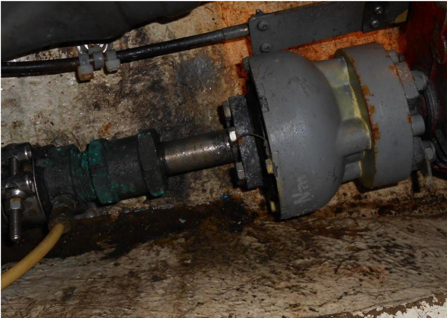
Centaflex M127 with spacer to allow easy removal
