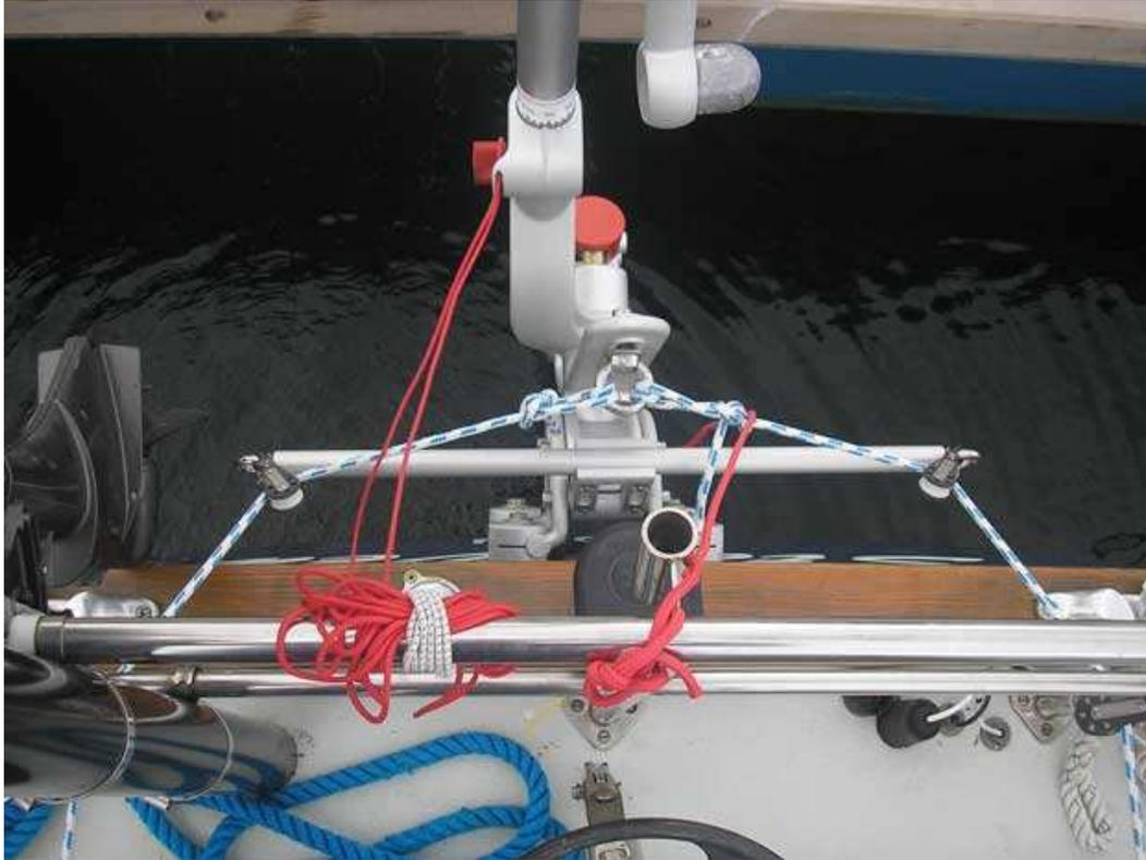
From the blocks on the extension bar the steering lines need to run through blocks attached to the lower rung of the push-pit and then onto blocks sitting each side of the tiller. At least one Contessa owner has modified the seat-back at the aft of the cockpit so that the lines can run directly from the windpilot to the tiller turning blocks, this was achieved by cutting some large holes and glassing in tubes that the lines pass through.
