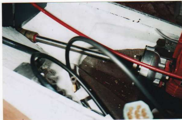
Figure 3 - PSS Shaft Seal & Centaflex Gearbox/Shaft Coupling. Note roll of red tape just visible in stern tube. With this set up you can put a short length (say 150mm) of bar into the coupling to align things with a steel rule across the two
