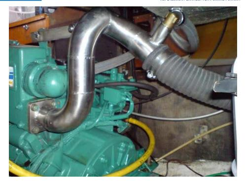
The new riser in place. The engineers tack welded it first but it was right first time. The new piece is lighter than the old cast elbow, but is a longer lever arm. To support it I used a short bar across to the engine lifting lug
