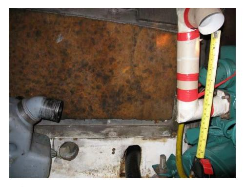
The prototype for the replacement exhaust riser. I want to raise it at least 6 inches - managed to get about 8 to close under the cockpit floor.
