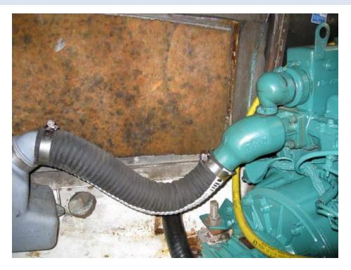
This is the old configuration. Not much fall from the mixing elbow to the water lock. I think the waterlock used to be slightly lower but only loosely affixed with cable ties, before being bolted to the cockpit locker side
