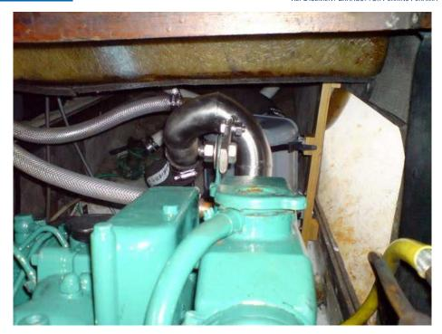
The waterlock is secured to a piece of wood bolted to the side of the cockpit locker. It also sits on a small plywood shelf expoxied onto the hull. The base is about 2 inches lower than the old waterlock
