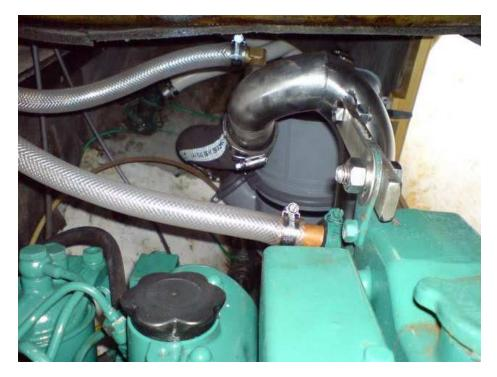
Behind the engine the gray cylinder is the new Vetus NLP water lock. It has 10 litre capacity in two chambers - 1 above the other
