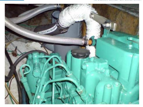
The new exhaust riser with lagging. Still some jobs to do - need a slightly longer water hose and a 2nd hose clip on the riser/pipe join. The engine now starts much more quickly and hopefully won't get any water into it again!
