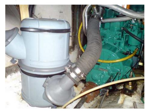
The waterlock. After use the lower part is left with about 2.5 litres of water and there is about 0.5 in the upper part. Each part has a drain plug. Since this picture I've fitted a hose to the lower drain which runs to the bilge. It can be accessed under the cabin floor to remove the plug and drain the waterlock
