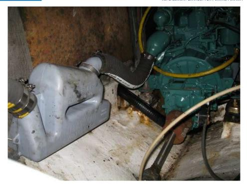
Another view of the old configuration. The waterlock capacity was 4.5 litres. When I went to remove it it was full almost to the top - probably about 4 litres. I think that this contributed to high back pressure and made it difficult to start
