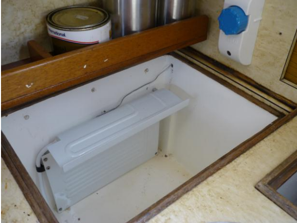
Refrigeration plate in the coolbox – just enough clearance to the lid Thermostat / off switch above
